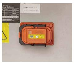
The electrical system is equipped with highvoltage interlocks, insulation detection and vehicle-grade safety means. The MSD maintenance switch enables one-click power-down and safer maintenance.
