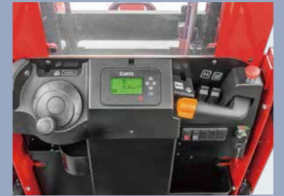
The FREE accelerator lever with sensor switch, as standard configuration, can prevent mis-operation during the work
